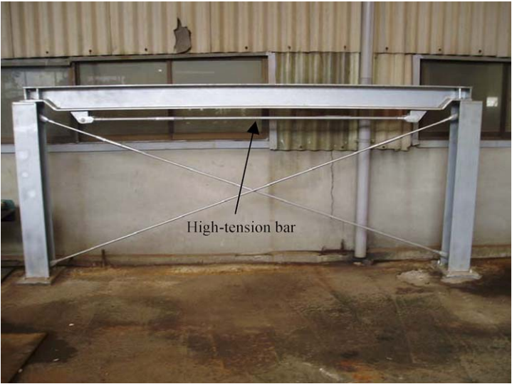
Fig. 3. A high-tension bar used in the laboratory experiment.
